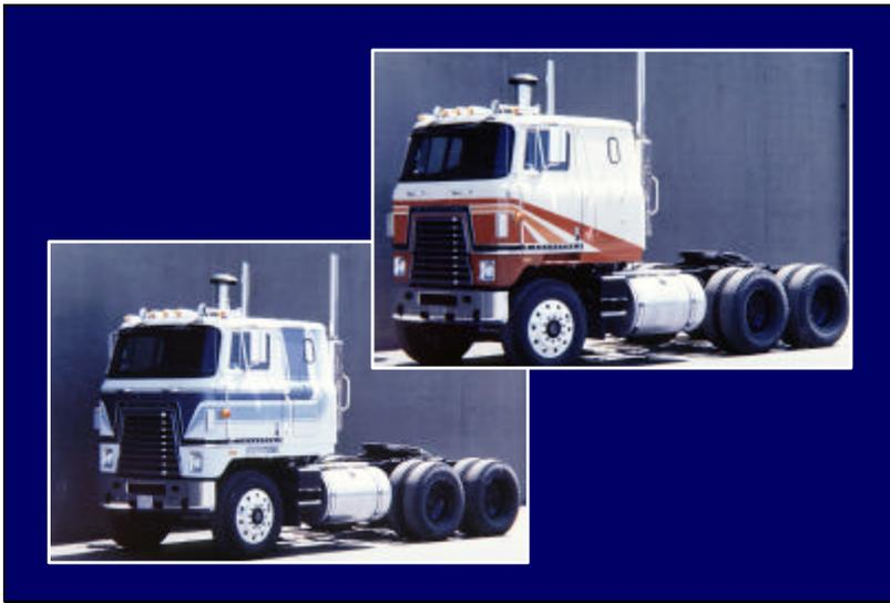
**Shown here are two identically spec'd (except for paint color) tractors that International contributed to the ride-demonstration project. One tractor towed a loaded trailer and the other an empty trailer to demonstrate the effect of cargo loading on ride performance.**
